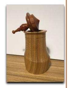
pression. The collar can be used to grip the tenon in the chuck and the live centre used for as long as possible to complete the finial. The finial can be any shape of your choice but, remember that the lower the centre of gravity of a spinning top, the better its performance. So, keep the finial simple to reduce the lid's overall weight and the top's CoG. You can now sand and finish the finial.
