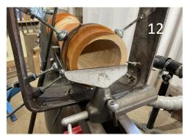
sten carbide cutters and, as the hole gets much deeper, my homemade chisel made from a steel pipe with another steel pipe welded into it, which takes the Roly Monro head (photo. 11). The insert of the pipe is filled with lead shot to give it weight and reduce vibration. It all works pretty well but is hard going as I wanted to get about 20" into the wood (photo. 12) before I could take it
