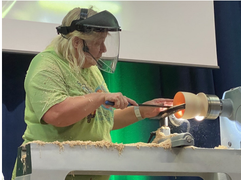
Joey Richardson demonstrates turning a thin-walled pot
