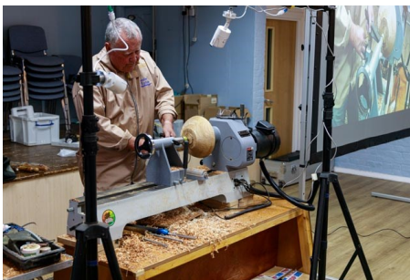
Shaping the outside - with sensible tailstock support
