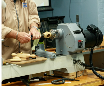
Making the female thread with a tap
