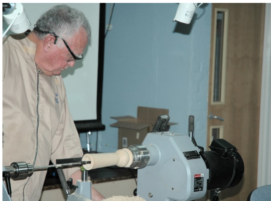
Boring out the main body of the mill
