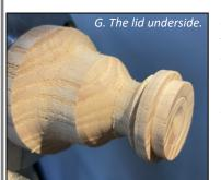
base. The tightness of this fit is your choice. The finial on my lid is delicate, so I chose a looser fit. Then you must make a shoulder on the bottom of the lid that fits into the hollowed hole of the base. The depth of the shoulder and the upper-
