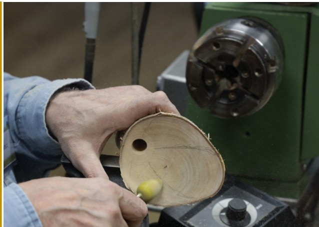
Using a carbide burr in a Foredom tool to embellish the top
