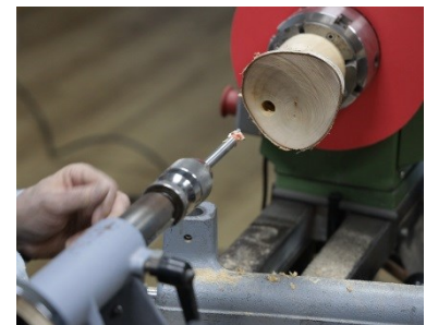
Drilling with a carbide-tipped Forstner
