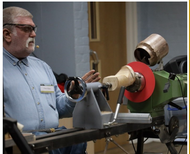
The work mounted ready for turning. The red disc shields the turner from the rotating counterbalance behind it.
