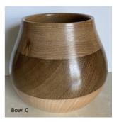
I have made layered bowls in the past, but I was sometimes discouraged by the phenomenon known as 'glue creep'. This happens when the glue fails to maintain a smooth join between the layers on the inside or outside of a finished bowl, resulting in one being able to feel a step in the join.
