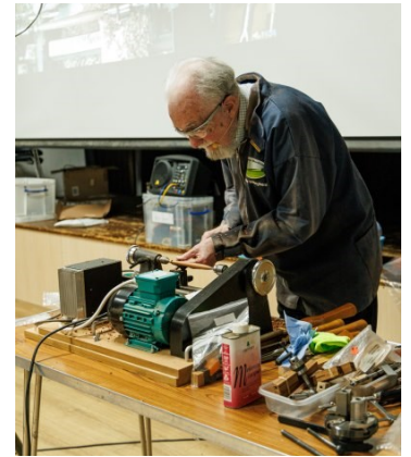
Norman turning a desk-top pen. The lathe is about a foot too low for his height and would lead to back problems if used that way!
